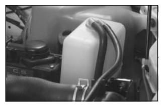
The coolant recovery tank is located toward the front of the engine compartment on the driver's side of the vehicle. See *Engine Compartment Overview on* page 5-12 for more information on location.
